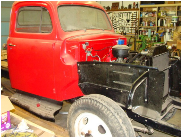
Ford F5 Medical Center farm truck. Front clip is sent out for a rebuild, wiring and exhaust completed. Next the truck is to be sent out for a paint job and the wood bed constructed.
