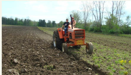
John Hartwick's Allis Chalmers 190XT with a 4 bottom semi mounted plow
