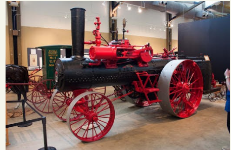
This Case Traction Engine is one of several steam engines to be seen at the museum and grounds. The steam engines at the wood shop, turpentine still, and saw mill are in operation when those demonstration areas are in operation. This Case is a focal point inside the museum where visitors can get up close to examine the boiler, firebox, engine components and controls.
